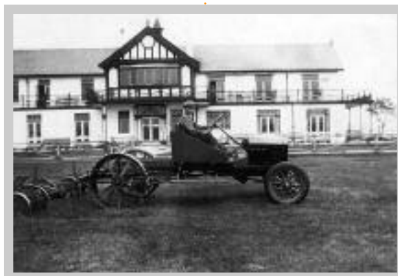
JP TAYLOR WITH THE NEW CAR CHASSIS FITTED WITH SPIKED STEEL REAR WHEELS TOWING GANG MOWERS IN 1923
